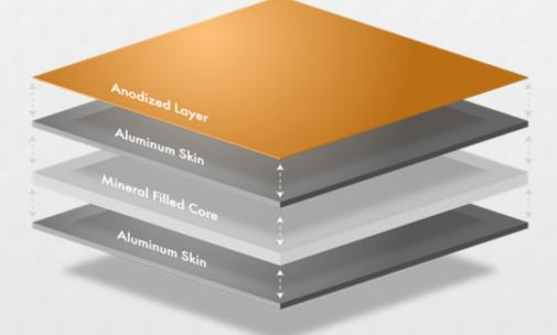
The anodizing process involves immersing the metal part in an electrolytic solution, usually sulfuric acid, while applying a current. This causes an oxide layer to form on the metal's surface through the oxidation of the metal itself. The thickness and properties of the oxide layer can be controlled by adjusting factors such as the voltage, current density, temperature, and duration of the anodizing process.
